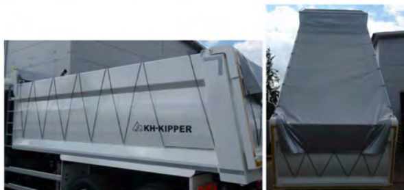
Fig. 28. Tarpaulin laid down in a correct manner.
