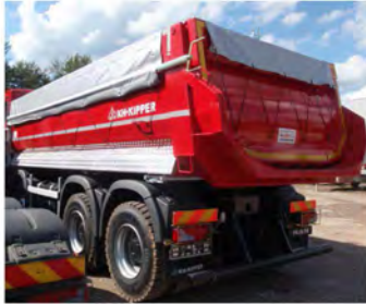
Fig. 31. Tarpaulin laid down in a correct manner
