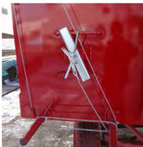
Fig. 25. Example of the way of securing the spare tyre rope.
