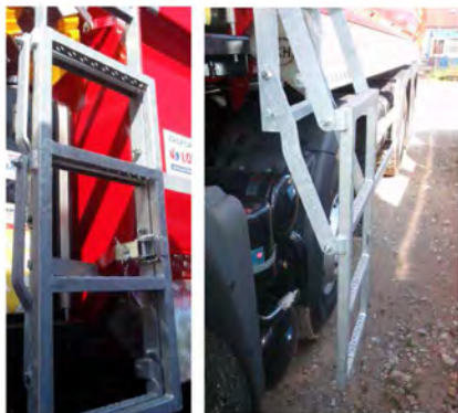
Fig. 27. The ladder on the front wall.
