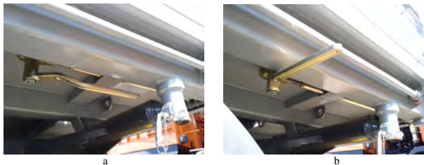
Fig. 7. The lever for opening / closing tailgate hooks; a) closed position, b) open position.
