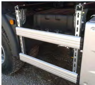
Fig. 33. Collision protection barriers
