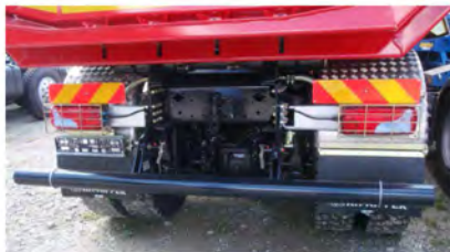
Fig. 35. Folding bumper in lowered position
