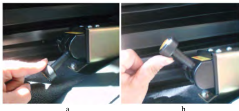
Fig. 10. Pneumatic control valve for the hydraulic gate: a) gate opening, b) gate closing.
