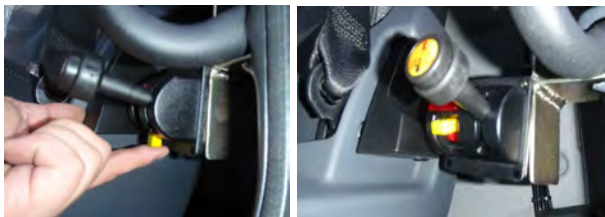
Fig. 9. Opening of the gate with the use of the switch integrated with the load bed lifting controller.
