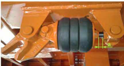
Fig. 38. Hyfix lock – example of fixing.
