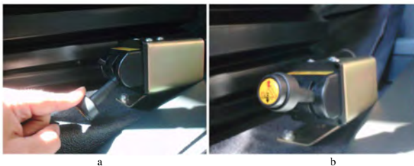
Fig. 21. Pneumatic valve which controls the load bed lifting and lowering: a) load bed lowering, b) neutral position.
