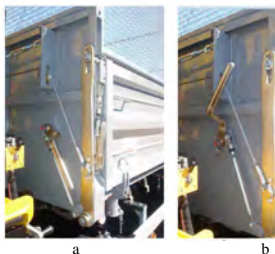
Fig. 17. Side gate lever: a) closed position, b) open position.
