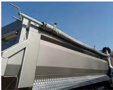
Fig. 26. Tarpaulin: a) rolled up to the front wall, b) rolled up to the side gate.
