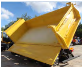
Fig. 15. Hydraulic gate opened for the purposes of unloading loose materials.
