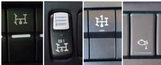
Fig. 5. Examples of switches and symbols of power take-offs.
