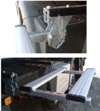
Fig. 34. Lifting of collision protection barrier
