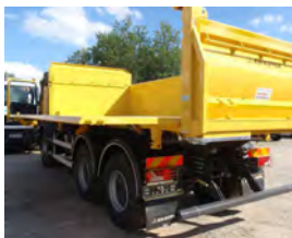
Fig. 15. Hydraulic gate opened for the purposes of unloading loose materials.
