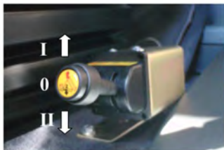
Fig. 20. Pneumatic valve which controls the load bed lifting and lowering: "I" load bed lifting; "0" – neutral position, "II" – load bed lowering.
