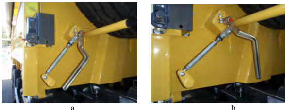
Fig. 8. The lever for opening / closing the side gate hooks: a) closed position, b) open position.
