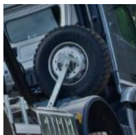
mounting of spare wheel on the frame
