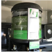
central greasing system
