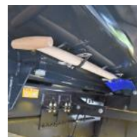
mounting a shovel under the floor
