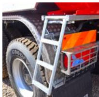
foldable ladder for operating the tarpaulin
