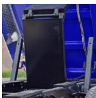
supporting legs under the body
