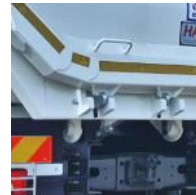
hook protection against damages
