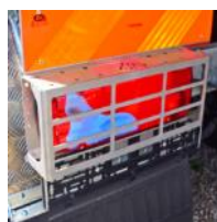
rear lamp covers with tiltable grill
