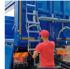
ladders and platforms enable entry on the body
