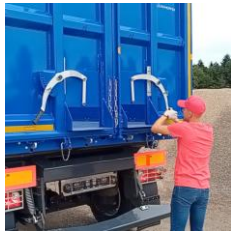
grain chutes enable precise unloading of grain
