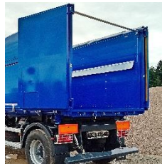
side-opening rear wall allows to load goods on pallets
