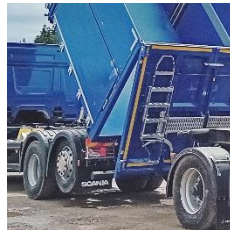
rear wall opens automatically when the body is lifted backwards
