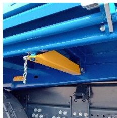
repair supports under body
