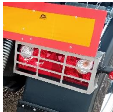
back lights steel protection with easy opening grate
