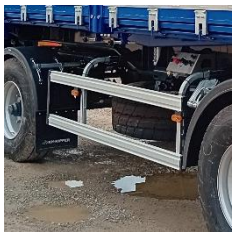
aluminum side underrun protection
