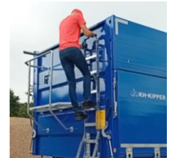
ladders and platforms enable entry on the body
