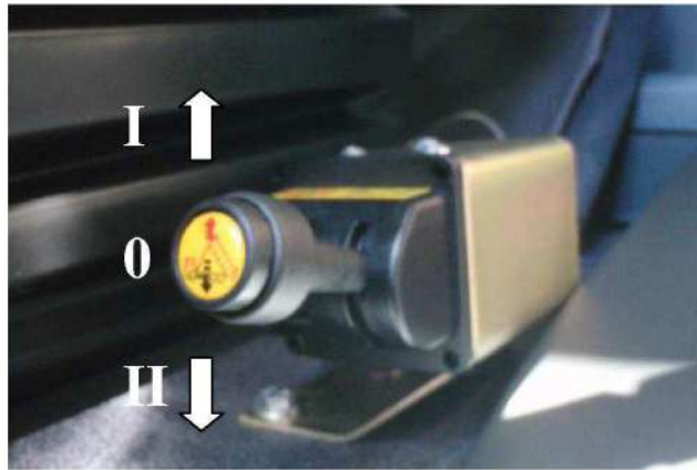
Fig. 12. Pneumatic valve which controls load bed lifting and lowering: "I" - load bed lifting; "0" - neutral position; "II" - load bed lowering.
