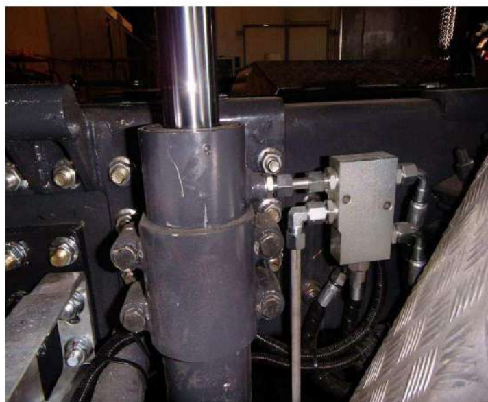
Fig. 42. Lifting / lowering servomotor.
