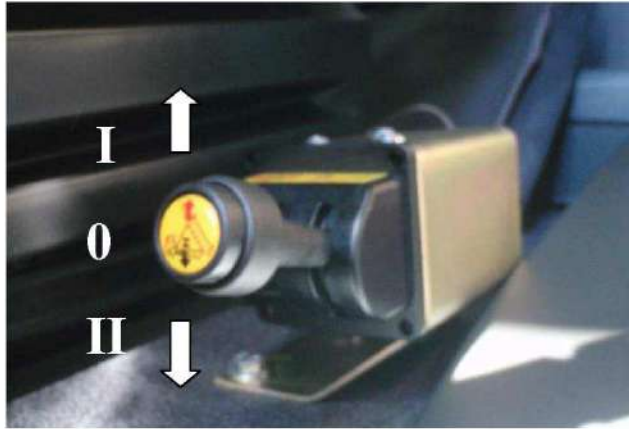
Fig. 14. Pneumatic valve which controls load bed lifting and lowering: “I” – load bed lifting; “0” – neutral position, “II” – load bed lowering”.
