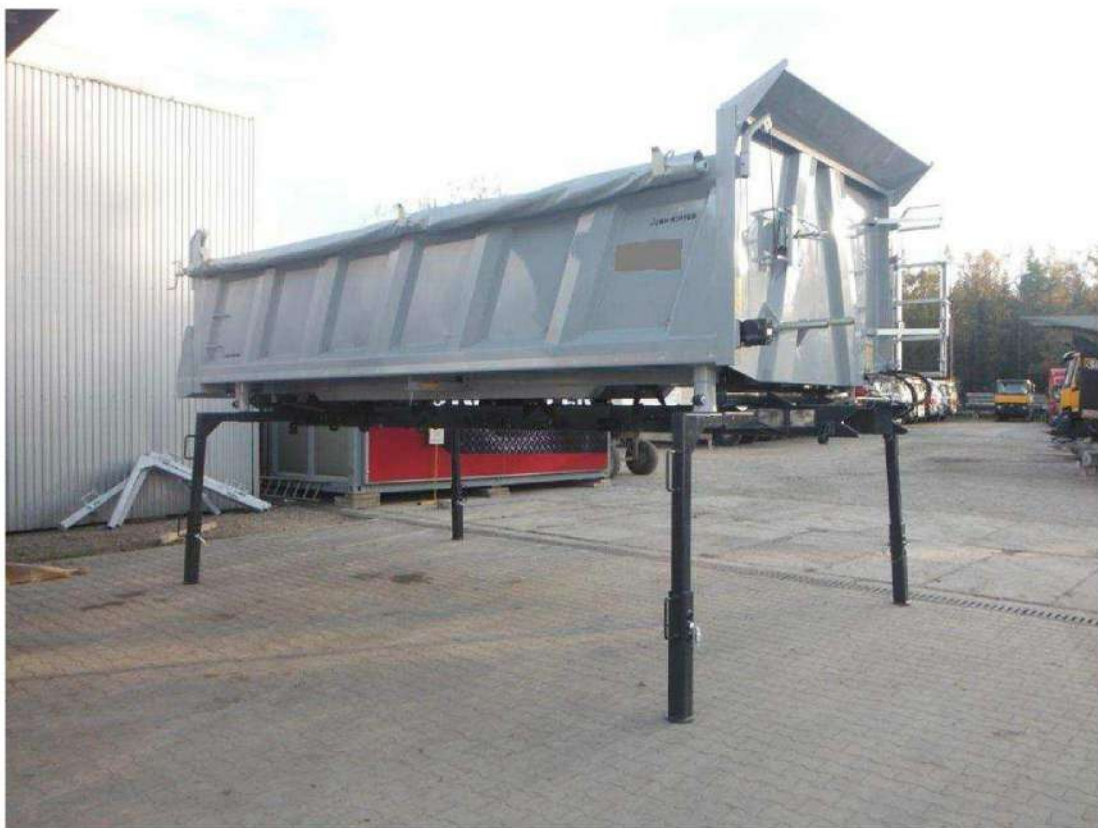
Fig. 40. Tipper load bed on side brackets.
