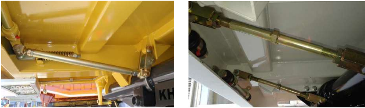
Fig. 6. Examples of tensions members for opening / closing of the tailgate.
