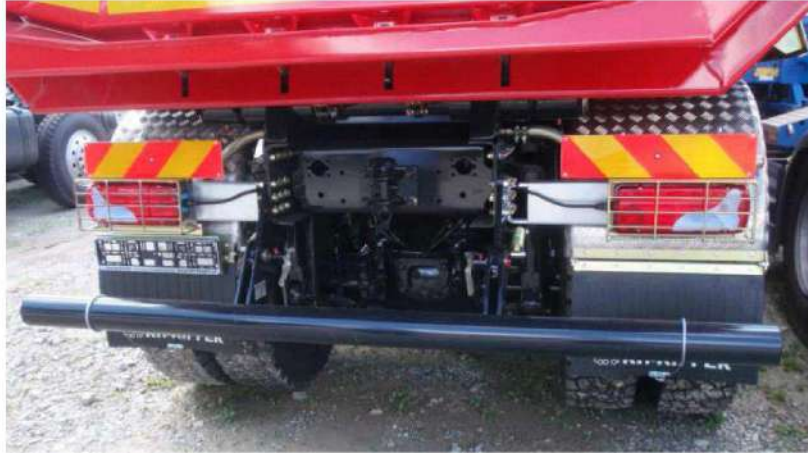
Fig. 35. Folding bumper in lowered position
