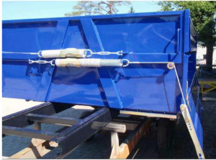
Fig. 19. Example of the spring steering system for the side gates.
