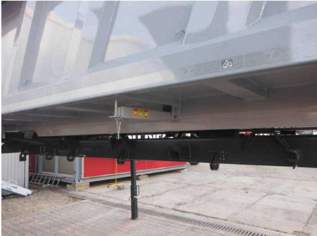
Fig. 41. Bodywork auxiliary frame bushings for locking on the chassis.
