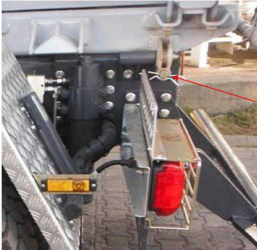
Fig. 47. Safety pin with a cotter pin. Locked bodywork.
