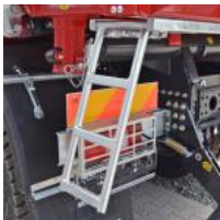
Folded ladder from under the floor to operate tarpaulin
