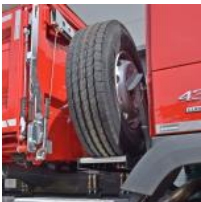
Mounting of spare wheel with winch behind cab
