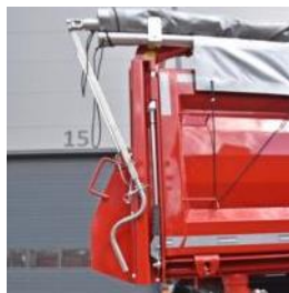
The crank and the poker hook for the lines can be folded when they are not used
