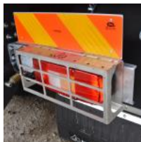
Rear lights protections with openable grate
