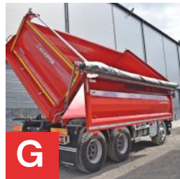
Unloading of the loose materials after releasing of the bottom locks
